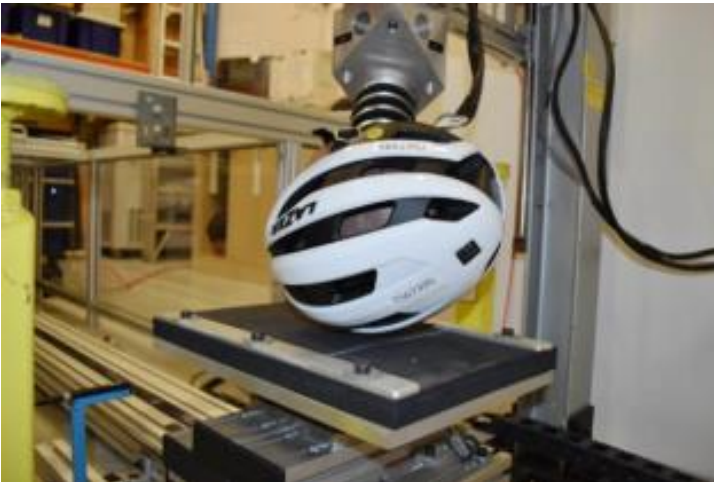
Figure 15: Helmet test set-up at Transport for NSW's Crashlab facility
