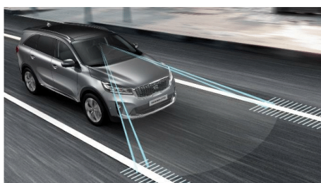
Figure 4. Illustration of camera detection used in Lane Keep Assist technology iv
